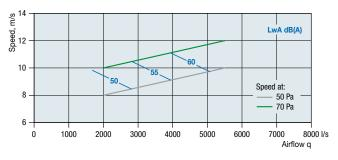
Correction of sound power level,  $L_{wok}$  in octave band  $L_{wok}$  (dB) =  $L_{wA} + K_{ok}$
